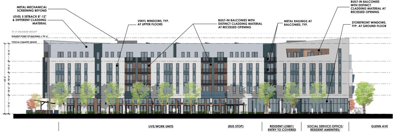
**1 NORTH ELEVATION (SHAW AVE FRONTAGE - 91.6% BUILDING COVERAGE)** \* MAX BUILDING HEIGHT PER FMC SECTION 15-2102 A, B & C.3 & SECTION 15-2103 A. SCALE: 1"=20'-0"
