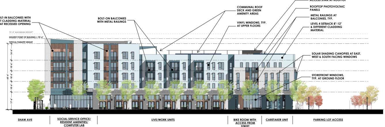
**4 WEST ELEVATION** \* MAX BUILDING HEIGHT PER FMC SECTION 15-2102 A, B & C.3 & SECTION 15-2103 A. SCALE: 1"=20'-0"
