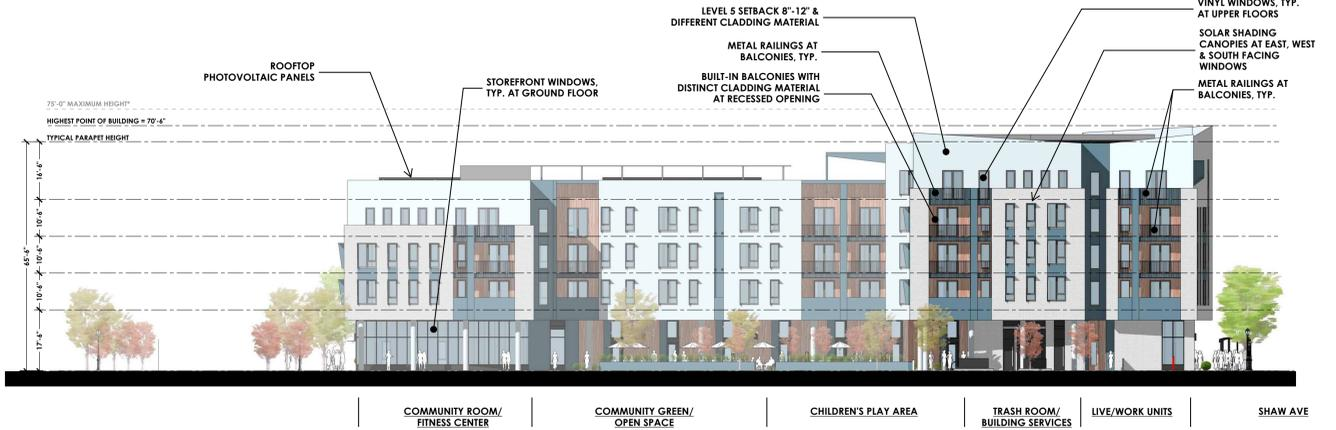
**2 EAST ELEVATION** \* MAX BUILDING HEIGHT PER FMC SECTION 15-2102 A, B & C.3 & SECTION 15-2103 A. SCALE: 1"=20'-0"
