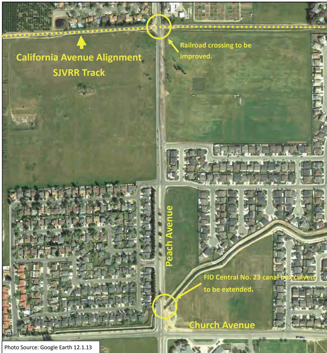
In order to develop Peach Avenue to the arterial street standard, additional right-of-way is needed from the undeveloped properties along Peach Avenue from Church Avenue north to the California Avenue alignment (San Joaquin Valley Railroad track)
