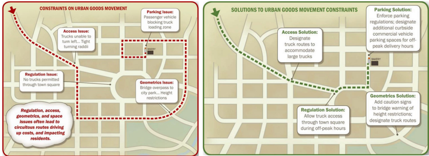
Figure 4.9: Examples of Truck Route Access
