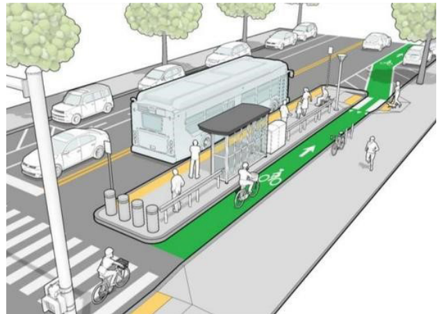
Possible resolution: bicyclists travel between a bus stop island and the sidewalk. Photo credit: Rhode Island Public Transit Authority
