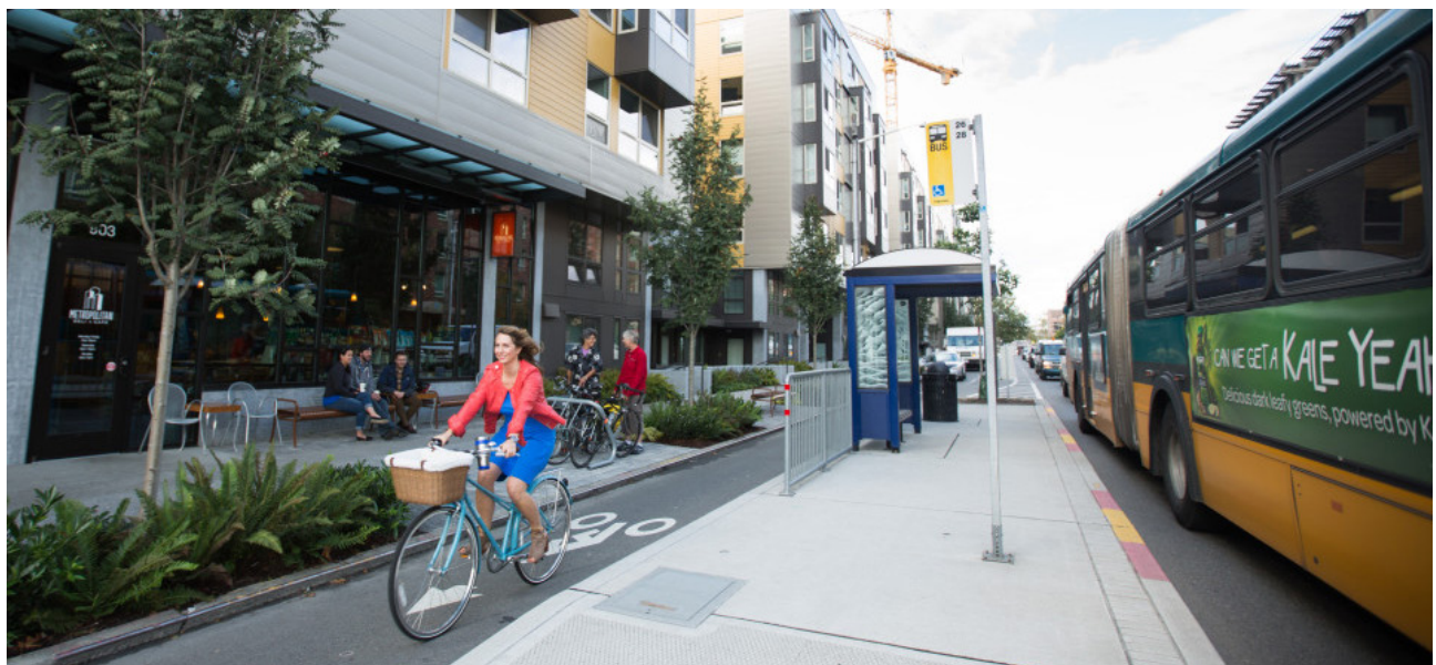
Protected bike lane behind bus boarding island. Photo credit: NACTO
