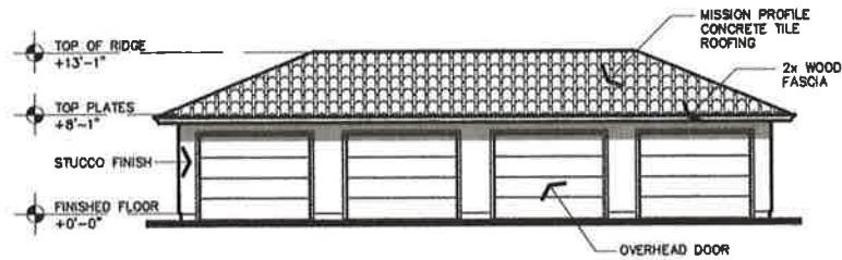
BUILDING G FRONT ELEVATION
