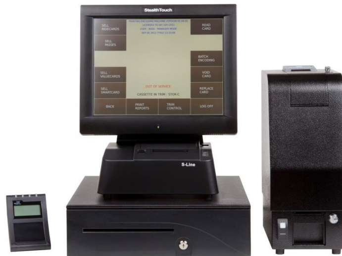
PEM printer/encoder machine – smart card reader at left, TRiM at right
