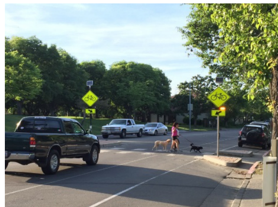
Figure 27: Rectangular Rapid Flashing Beacons in Davis
