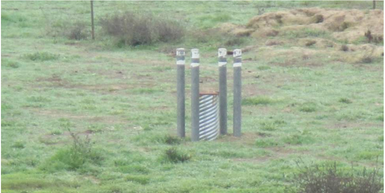
Photo 18: Groundwater Monitoring Well
