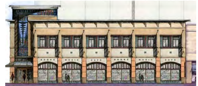
Storefront Bays. This building shows a human-scaled division of a street-level façade into a series of storefront bays.
