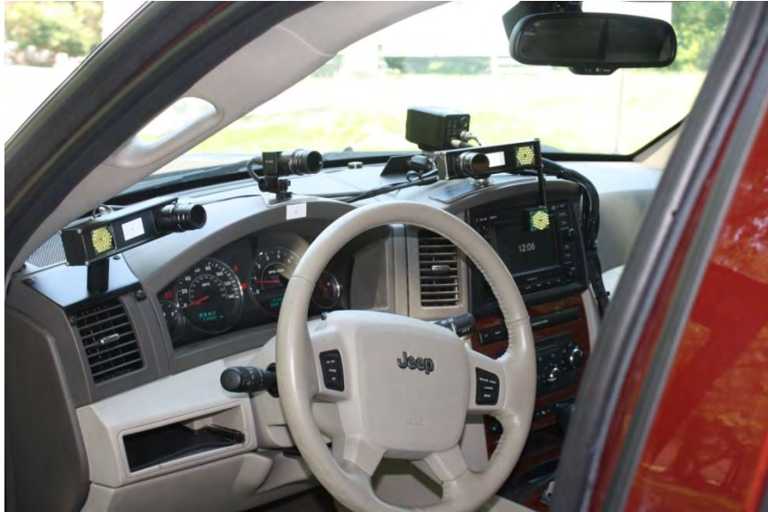
Figure 1. Eye tracking system camera placement.
