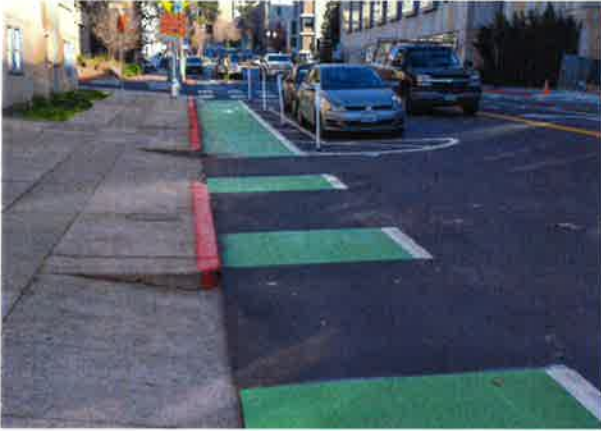
Figures 3.22: Bikeway-Driveway mixing zone
