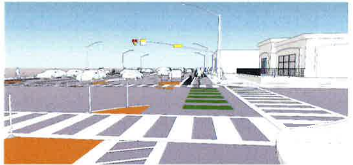
Fig 3.13: Example of soft-hit posts as curb-extensions, median-refuges
