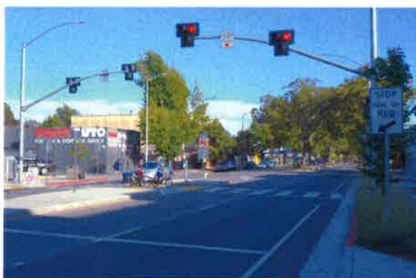
Figure 3.9: A Pedestrian Hybrid Beacon (PHB) in Albany, CA
