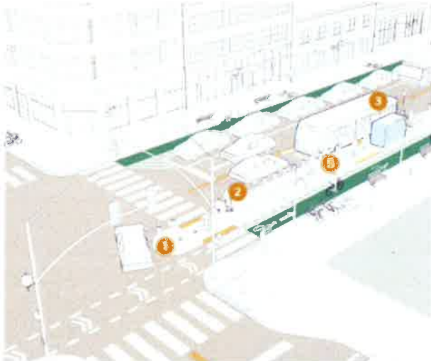
Figures 3.23: Bikeway at Bus Stop Areas (Source: NACTO Transit Street Design Guide)
