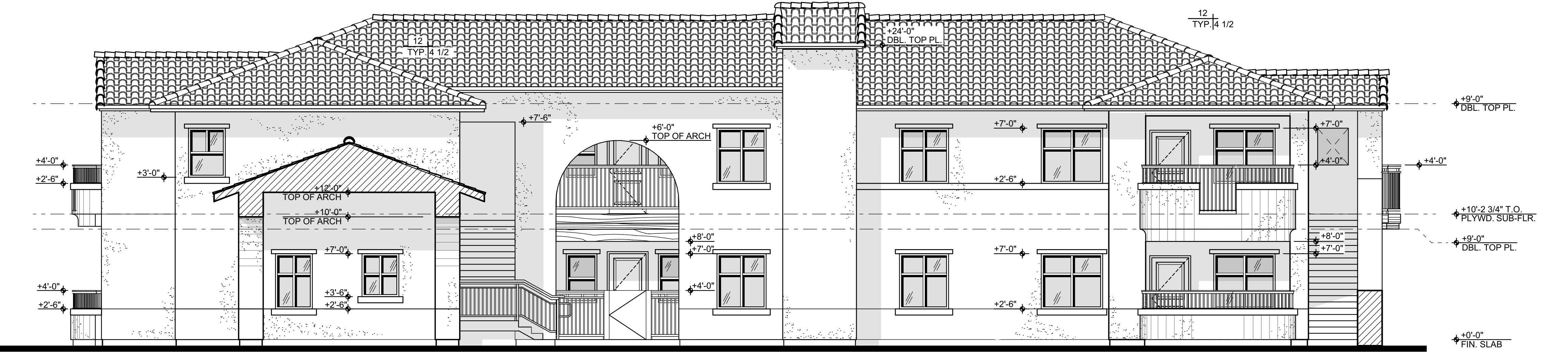
BUILDING TYPE '1' - COURTYARD ELEVATION SCALE: 3/16" = 1'-0"
