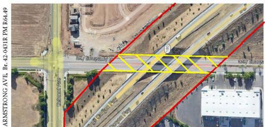
EXHIBIT A Armstrong ave. br. 42-0431L PMR64.47 RIGHT OF WAY LINE RIGHT OF WAY LINE AREA TO BE MAINTAINED BY CITY (INCLUDING SIDEWALKS AND CURB RAMPS)
