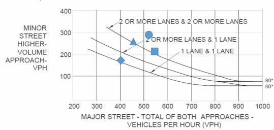
\*Note: 80 vph applies as the lower threshold volume for a minor-street approach with two or more lanes and 60 vph applies as the lower threshold volume for a minor street approach with one lane.
