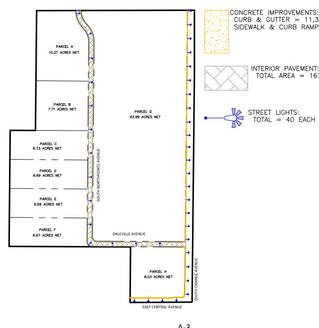
CURB & GUTTER = 11,325 LF SIDEWALK & CURB RAMPS = 24,028 SF
