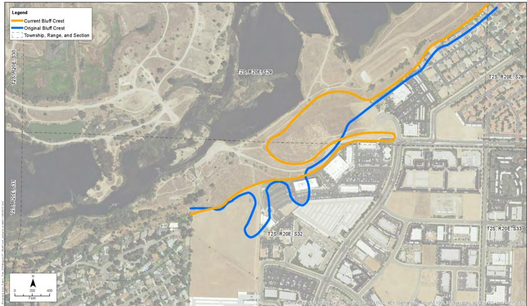
Figure 1-2 Conceptual Outline of the Original Bluff Crest (circa 1937) vs Current Crest
