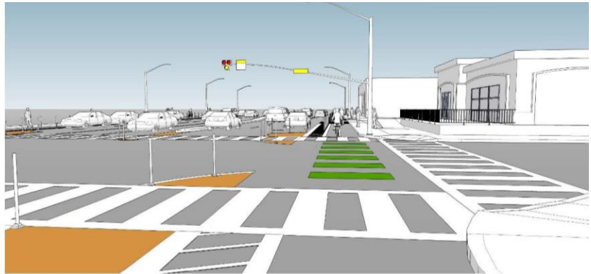
Fig 3.13: Example of soft-hit posts as curb-extensions, median-refuges
