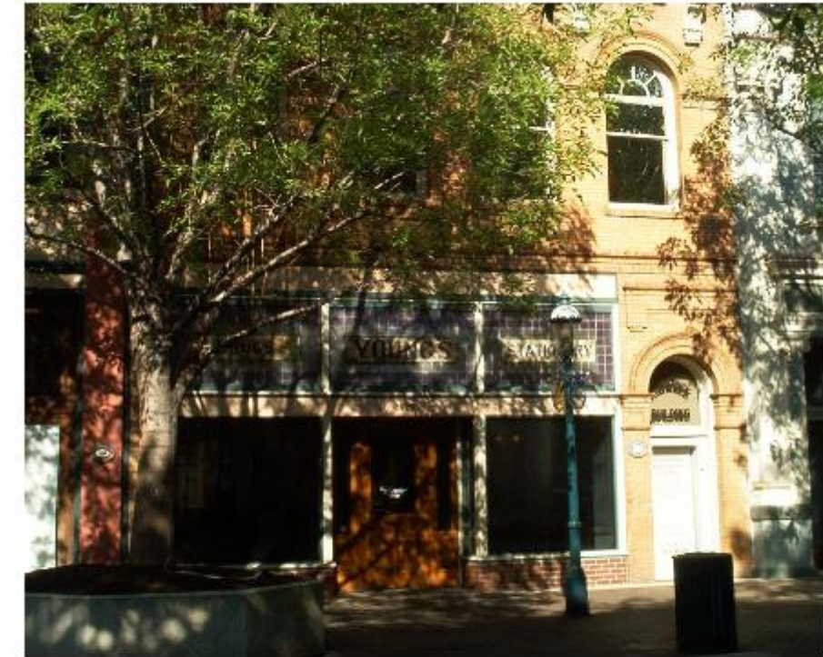
Separated Residential and Retail Entrances. This small mixed-use building has separate entrances for retail (left) and residential (right) components.
