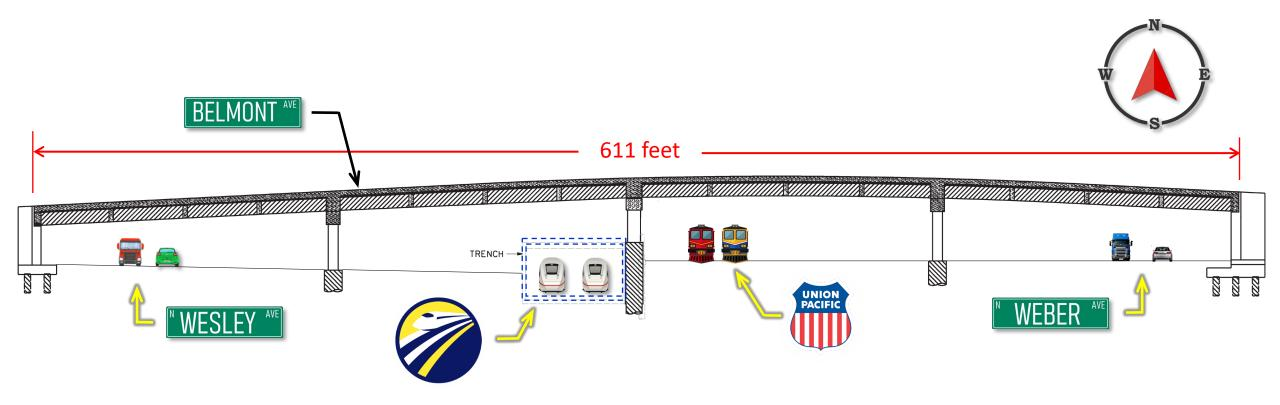
The proposed bridge is a four-span structure with a total length of approximately 600+ feet and a width of 64 feet. The bridge deck will consist of PC/PS concrete girders supported by a multiple column bents and short-seated abutments founded on 3-foot diameter Type I CIDH piles located within wrapped around MSE walls.
